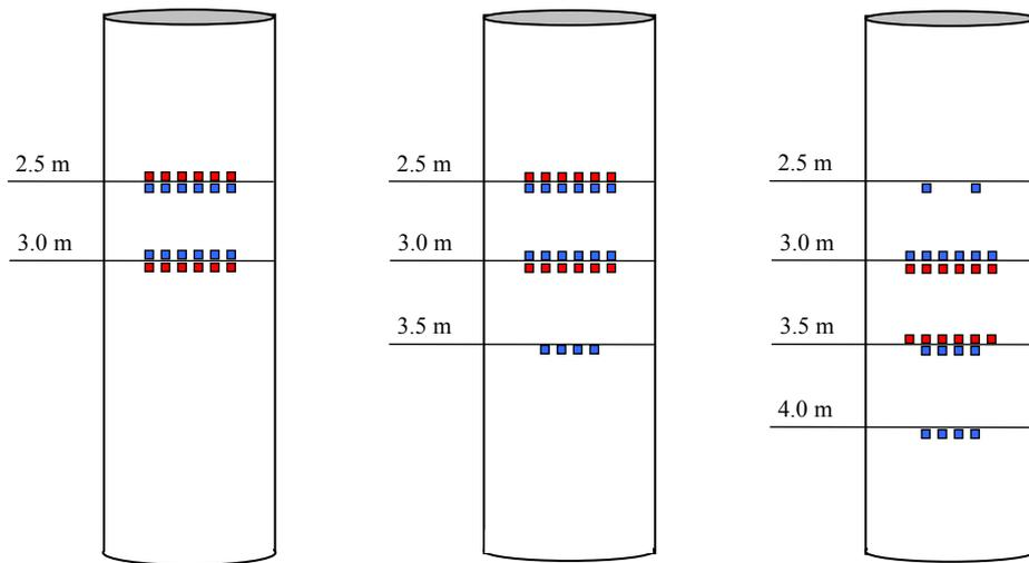
**Figure 3-6** The complete measurement position layout, both short and wide range LVDT sensors. Blue indicates a short range sensor and red a wide range sensor. The left setup is the original, the middle shows the setting after 2004 June 03, and the right one the setup after 2004 June 17.
