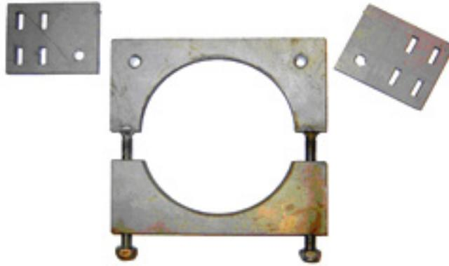
**Figure 5-9** The sensor fastening device. The device can be moved up and down the pipe in order to find a good measuring position before it is securely fastened to the pipe. The sensors can also be individually adjusted sideways. The device can hold up to four sensors.
