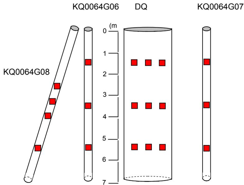
**Figure 3-2** The vertical layout of the thermocouples in the boreholes. Since the layout in the large holes are identical, only one of the two holes is shown. The sensors were positioned at 1.5, 3.5 and 5.5 meter down the holes. The exception is the KQ0064G08 hole, far left in the figure, in which the sensors measured the temperature at 2.75, 3.25, 3.75 and 5.5 meters. All depths are given relative the tunnel floor at -446.07 metre level.
