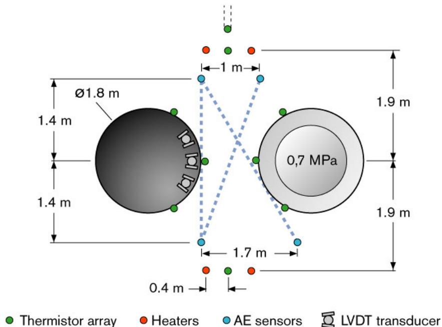
**Figure 1** The experiment geometry seen from above. The open hole to the left is illustrated with the pipe construction and LVDT sensors, to the right is the confined hole. The temperature, heater and acoustic emission (AE) holes are also marked in the figure.
