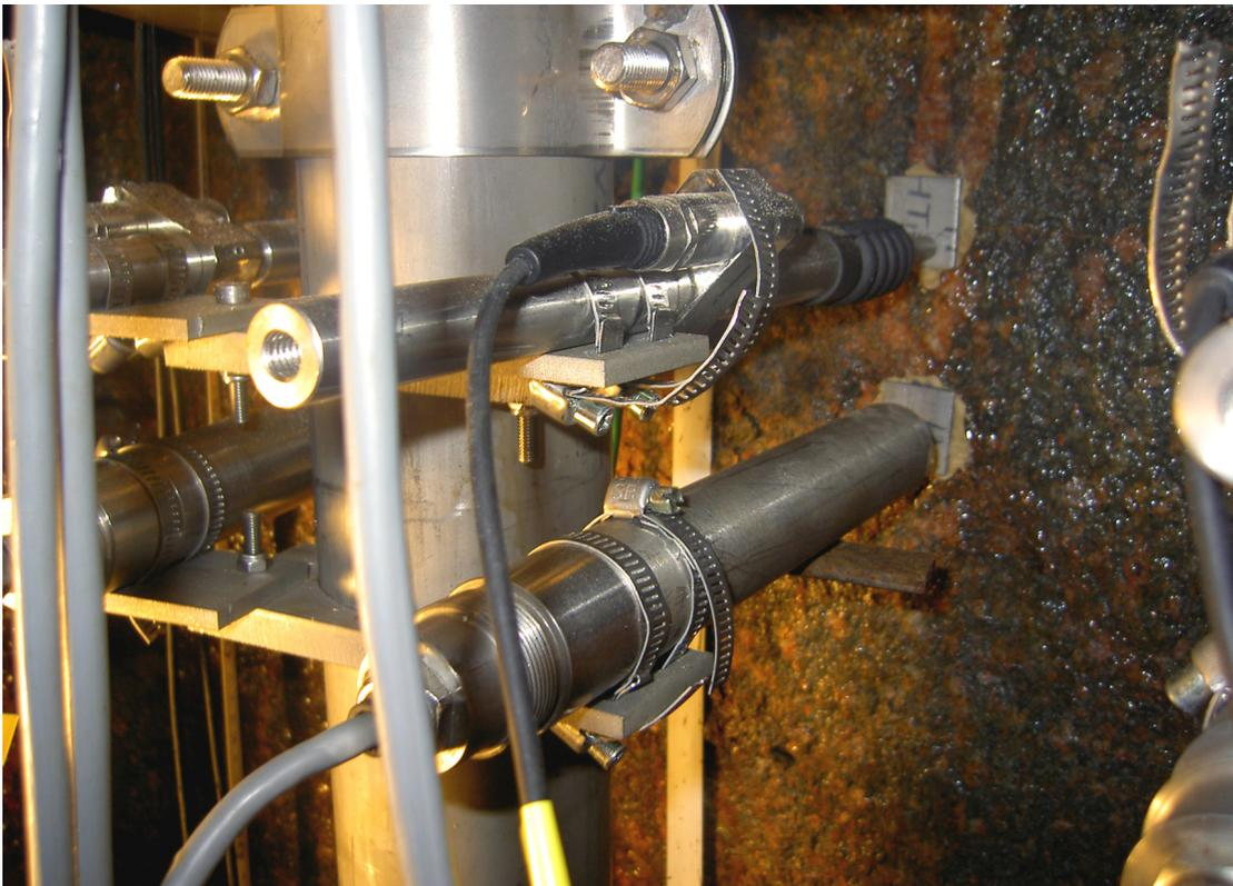
**Figure 5-10** The original clamp construction. As seen in the image both sensor types are secured using the method.
