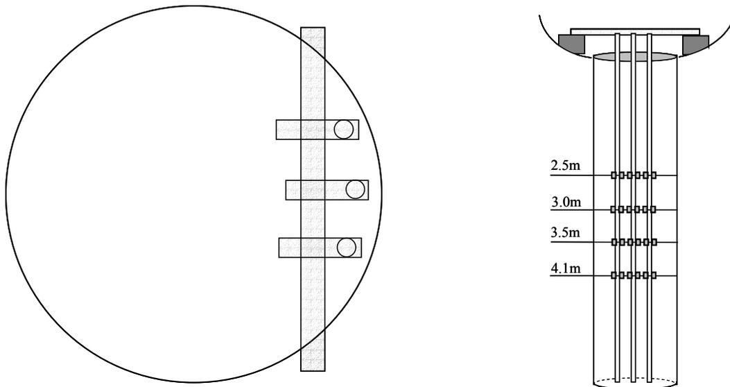
**Figure 5-3** Arrangement of the top crossbar used to stabilise the pipes in plan and section views. To the right the sensor levels with specified depths are also shown.
