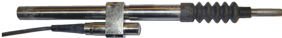
**Figure 2-3** The wide range LVDT sensor. The sensor has a range of 40 mm and the sensor output is 4-20 mA.
