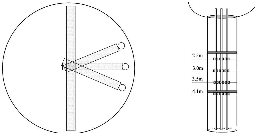
**Figure 5-4** Arrangement of the mid hole crossbars used to stabilise the pipes in plan and section views. To the right the sensor levels with specified depths are also shown.
