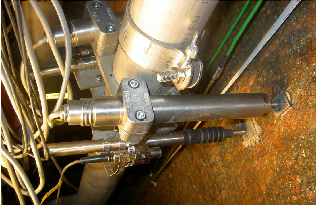
*Figure 5-11 The new clamp that was used to secure the short range sensors. As seen the wide range sensors are not fitted with the new clamp.*
