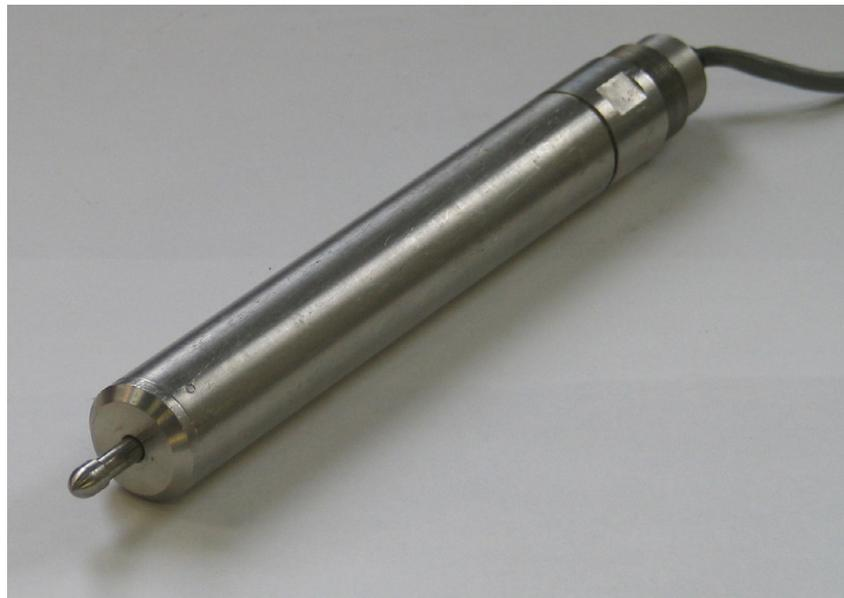
*Figure 2-2 The short range sensor mounted in the casing that protects it from dirt and water.*
