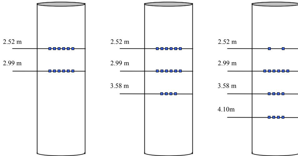
**Figure 3-4** Position map of the short range LVDT sensors in DQ00G3G01. The left setup is the original, the middle shows the setting after 2004 June 03, and the right one the setup after 2004 June 17.
