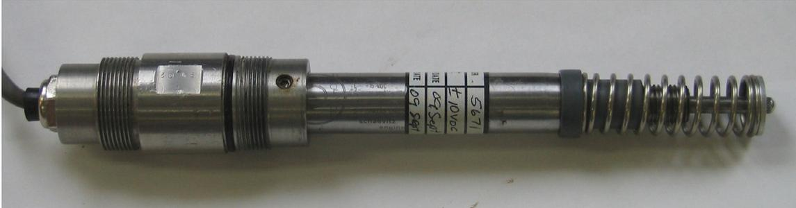
*Figure 2-1 The short range LVDT sensor without its casing.*
