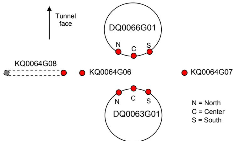
**Figure 3-1** The positions where the thermocouples are placed. The N, C, S markings are used to separate the positions within the same hole. Several sensors are placed below each of the marked positions.
