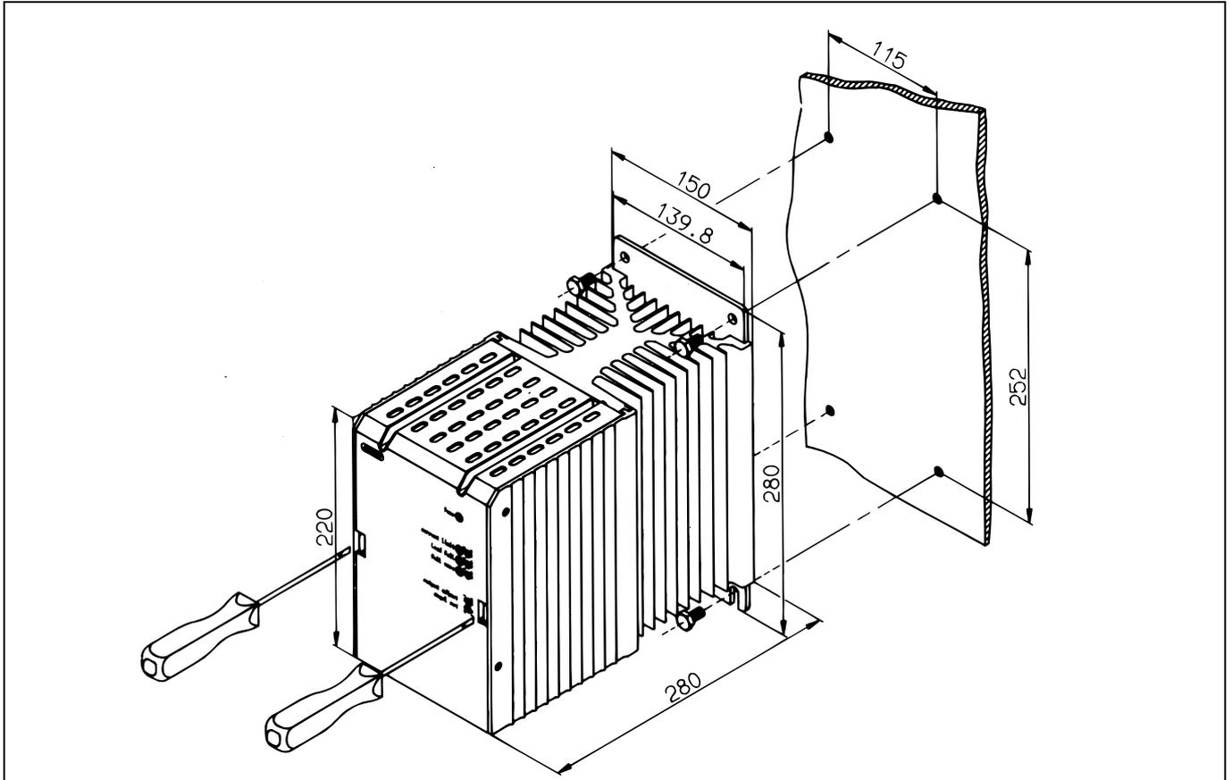
Mounting on rail to EN 50 022, or wall mounting for thyristor units up to 100 A
