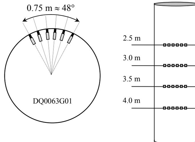
**Figure 3-3** To the right all potential LVDT sensor positions are displayed. Note that all positions were not used at the same time. The positions are marked as grey squares on the right image, the depths below the tunnel floor are also displayed. On the left the sensors are drawn from above to illustrate their radial positioning.
