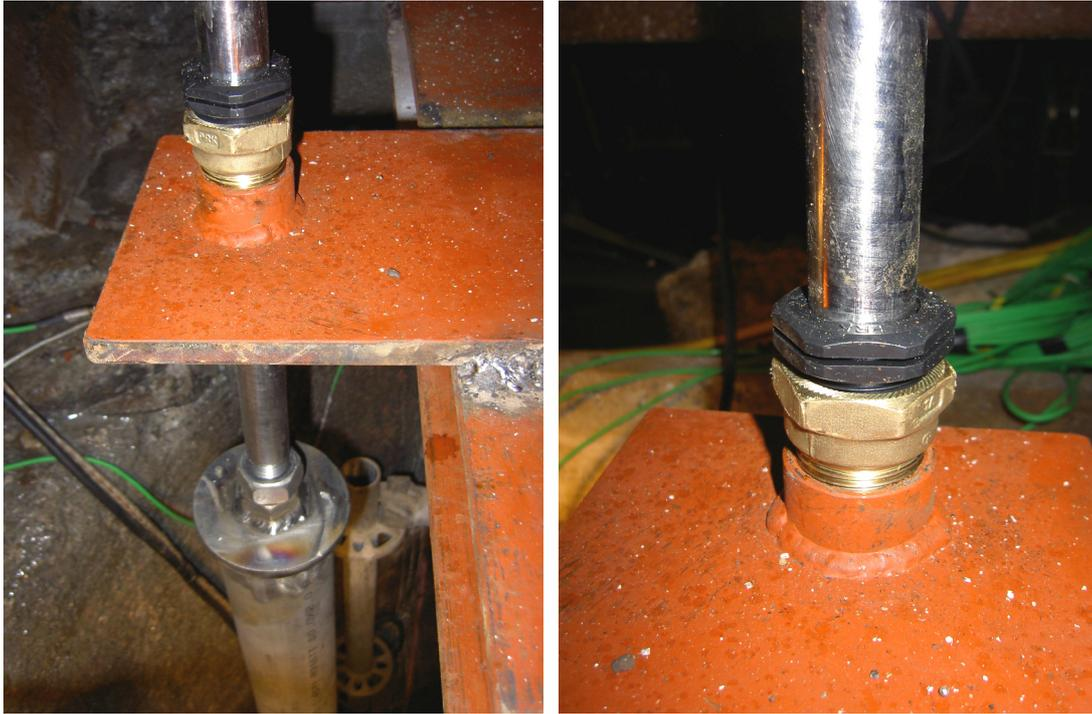
*Figure 5-7 Close-up's on one single plate with the coupling holding the pipe.*
