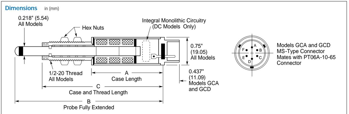
**GCA Specifications @ 2.5 kHz – AC-Operated Models**
