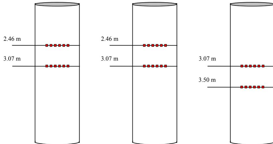
**Figure 3-5** Position map of the wide range LVDT sensors in DQ0063G01. The left setup is the original, the middle shows the setting after 2004 June 03, and the right one the setup after 2004 June 17.
