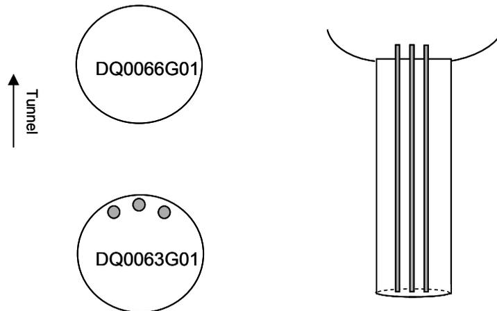
*Figure 5-2 Pipe Arrangement, in plan and section view.*
