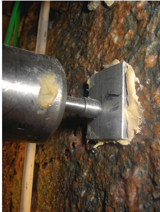
*Figure 5-12 One of the small steel plates glued to the pillar wall. A short range LVDT is mounted and using the plate as a measuring point.*
