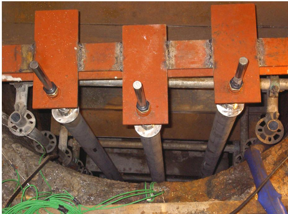
**Figure 5-6** *The plates on the top crossbar. The image shows the complete setup with the pipes in place.*
