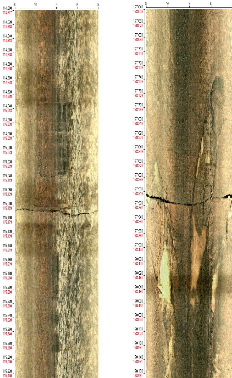
Figure 1-9. BIPS-images from KFM01A showing the probable main water-conducting open fractures from borehole sections 110–120.77 m and 176.8–183.9 m.
