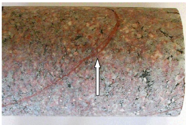
Figure 1-29. Fracture filled with adularia that is brick coloured due to micrograins of haematite. Some calcite is also present in the fracture. The diameter of the drill-core is approx. 5 cm. (KFM03A: 184.34–184.50 m).
