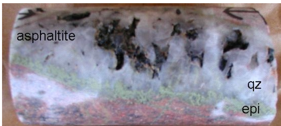
Figure 1-30. Drillcore with quartz and containing large voids partly filled with asphaltite (KFM01B: 2.97–23.05 m).
