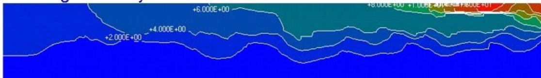
Figure 4-63. Computed tritium concentrations (simulated year 2004) using different values of recharge flow rate: a) 10 mm/year; b) 2 mm/year; and c) 1 mm/year. The transect coincides with the SW-NE cutting plane shown in Figure 4-2. The depth of the model domain is 1,000 m.
