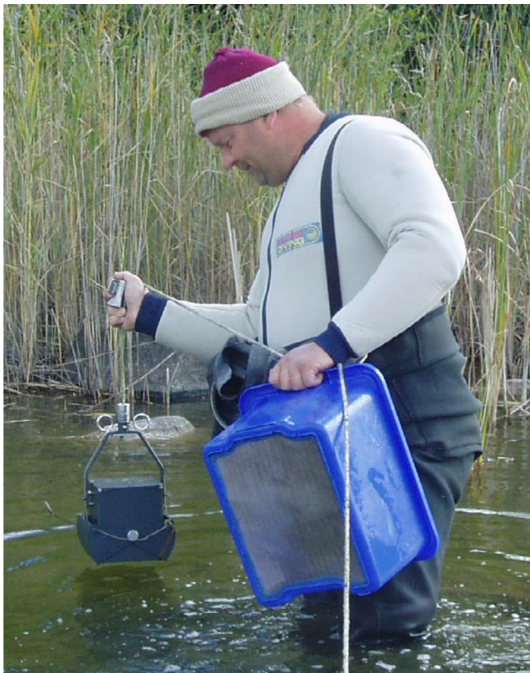
Figure 3-1. Sampling with an Ekman grab sampler.
