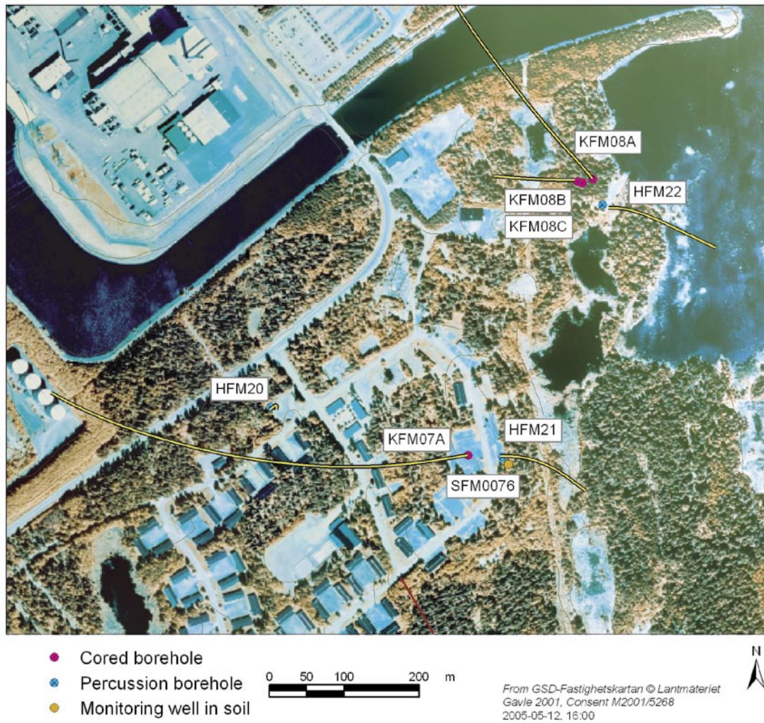
Figure 1-2. Borehole locations at and near drill site DS7. Besides the core drilled borehole KFM07A, the area comprises a monitoring well in bedrock (HFM21), and a monitoring well in soil (SFM0076). The projection of inclined boreholes on the horizontal plane at the ground surface (top of casing) is shown in the figure.
