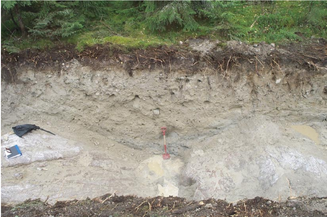
Figure 5-2. The deepest part of the trench LFM000810. The grey sediment in the bottom represents Unit B, clayey sandy silty till, overlain by the brown till representing Unit C.
