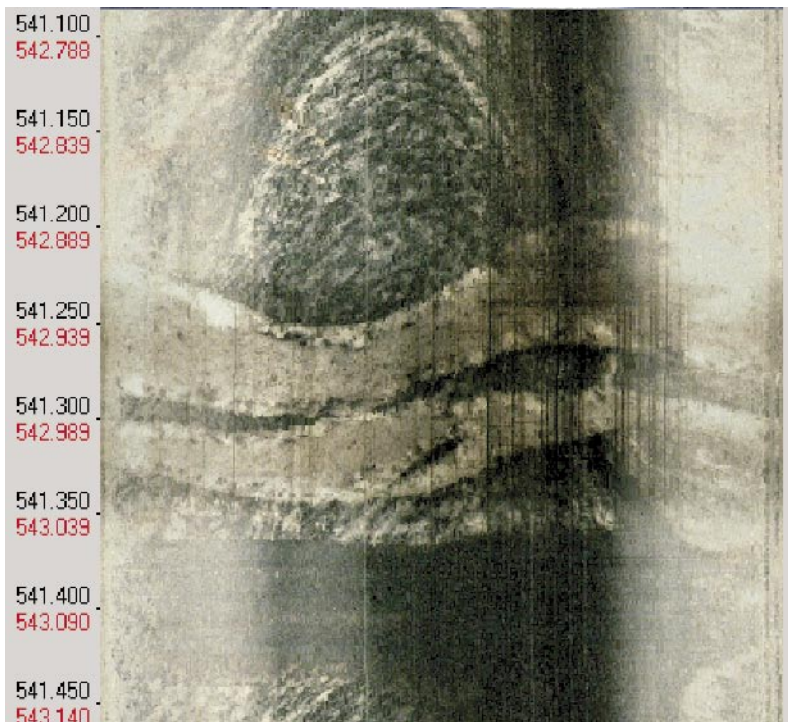
Figure 5-2. BIPS-image from the length interval 542.77–543.15 m of KFM07A, illustrating a high-strain zone cut by two veins of aplites (rock code 1062). Note the two fractures with oxidized walls visible in the upper left part of the image.
