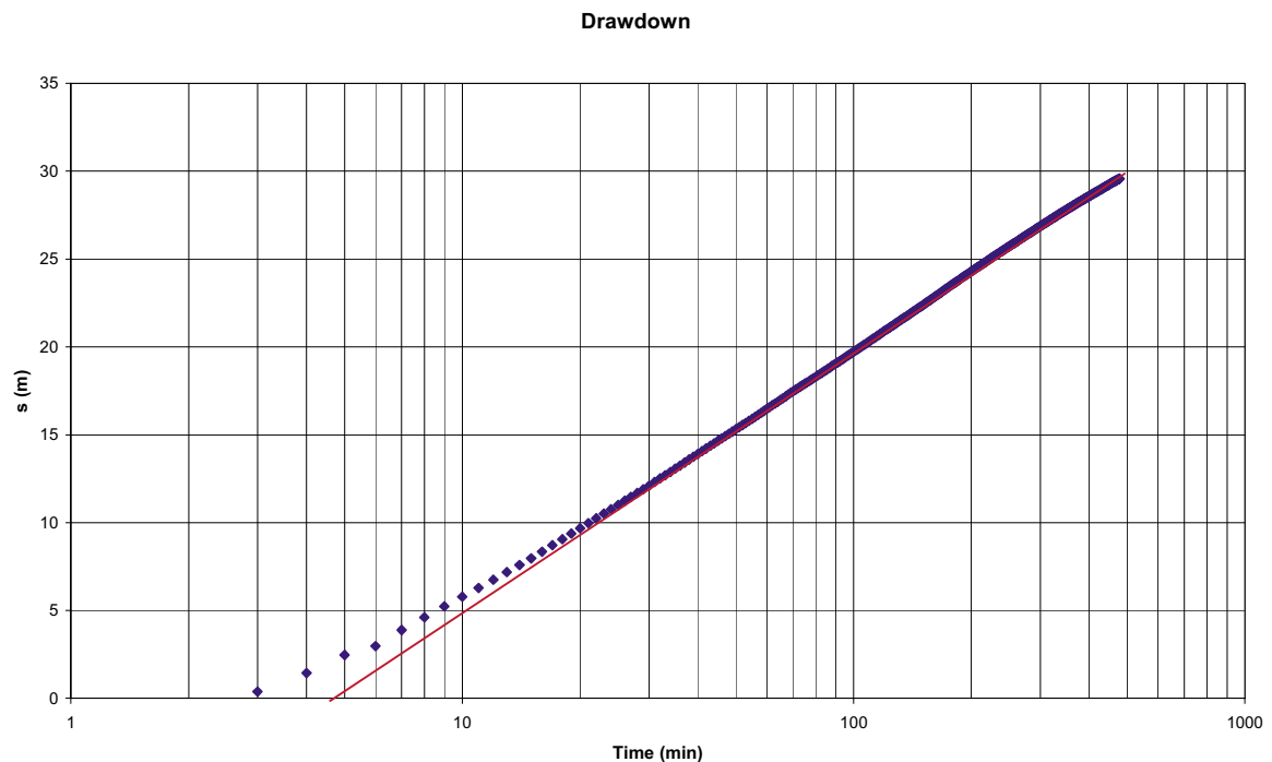
Figure A3-1. Drawdown in HLX18. The pumped flow, Q , was 60 litres per minute or 1.0 \times 10^{-3} \text{ m}^3/\text{s} . The drawdown, \Delta s , over one logarithmic cycle (between 10 and 100 minutes) was 14 m.
