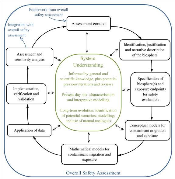
Figure 1. Schematic illustration of the enhanced BIOMASS methodology (in black) showing integration with the overall safety assessment (in blue) and the central role that is played by understanding of the disposal system (in green).
