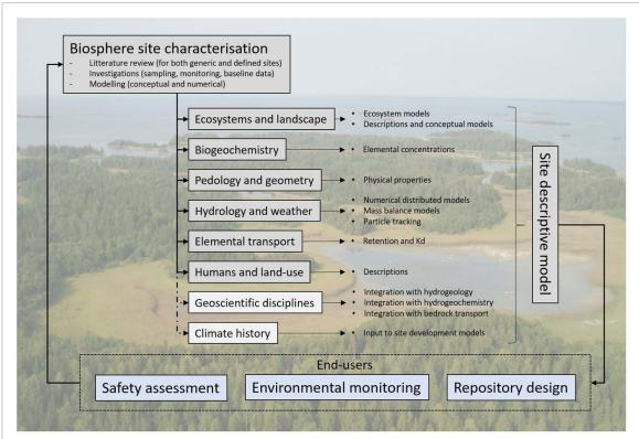
**Figure 3.** Illustration of a typical biosphere site characterisation setup in recent national radioactive waste repository programmes. Background photograph with permission courtesy of SKB.
